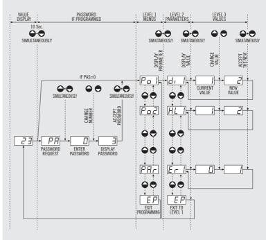
NOTE: If no key is pressed for 25 seconds in either of the previous steps, the controller will automatically return to the VALUE DISPLAY status without modifying any of the parameter
